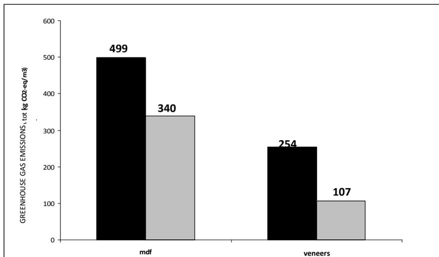
**Figure 1:** Comparison of emissions (kgCO<sub>2eq</sub>/m<sup>3</sup>) between conventional MDF panels (in black) and banana fibre panels (in grey), and wood fibre veneers vs Beleaf veneers
