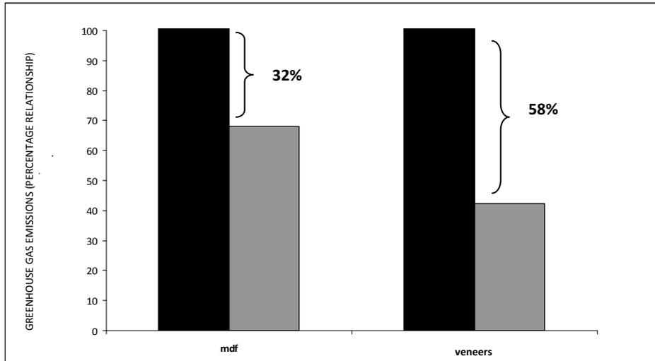
**Figure 2:** Comparison of emissions (%) between conventional MDF panels (in black) and banana fibre panels (in grey), and wood fibre veneers vs BELEAF veneers
